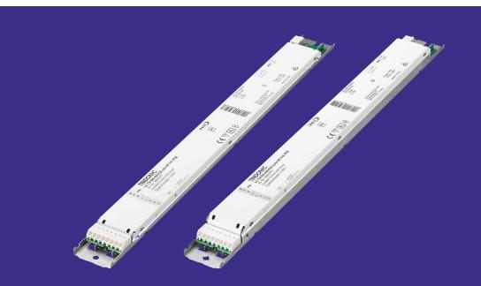
The new dimmable 16 mm or even 11 mm low profile drivers enable even more freedom in luminaire design while offering the same high technical standard as all Tridonic PREMIUM drivers such as low flicker and 1–100% dimming. The new NFC interface allows wireless programming during production. An integrated 14 V DALI power supply allows for a new way of sensor integration (16 mm only).
